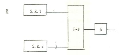
This is an arrangement  $\underline{A}$  except for the alternator (denoted by A) after the flip-flop. The alternator eliminates alternate bits.
