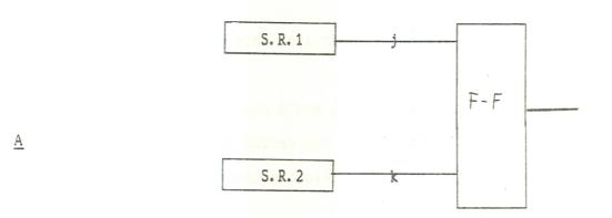
In this arrangement, there are two shift registers denoted by S.R.1 and S.R.2 whose outputs constitute the j and k inputs to a J-K flip-flop. We here consider S.R.1 and S.R.2 to generate maximum length shift register sequences. This whole arrangement is considered as generating a key sequence K which it can do once initializing vectors are input into S.R.1 and S.R.2. Clearly changing either S.R.1 or S.R.2 results in a new key.
