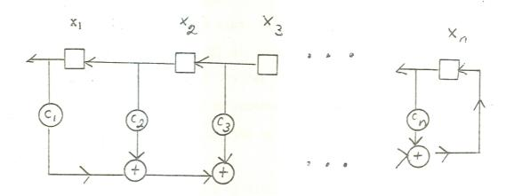
The figure above is a diagram of an n-stage linear shift register with feedback, for brevity we will just call this a shift register for the rest of this paper. Each of the squares labelled  $x_1, x_2, \ldots, x_n$  contains either a 0 or a 1.
