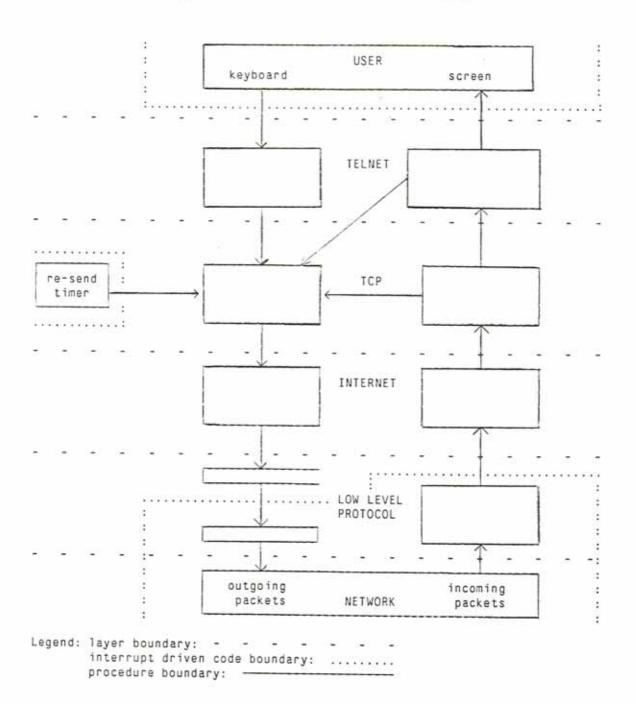
Internet between the time Telnet gets a character from the user and the time that it awakens TCP to send the character, then Internet will run after Telnet but before TCP. (The low level protocol processes packets coming off the net at interrupt level.) Running Internet between Telnet and TCP can result in unnecessary delay in sending the data that the user types.
