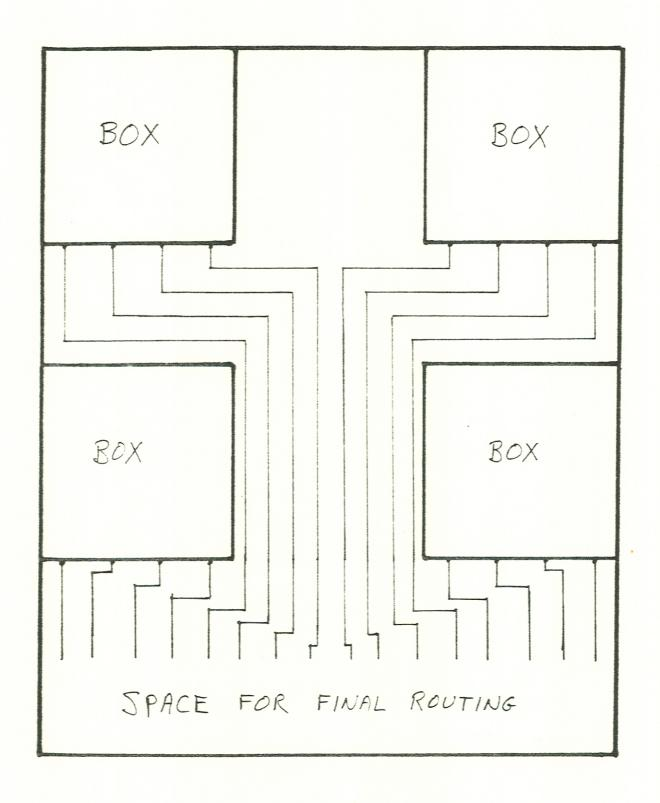
Figure 6. A view from above of the coalescing of the wires from the subgraphs.
