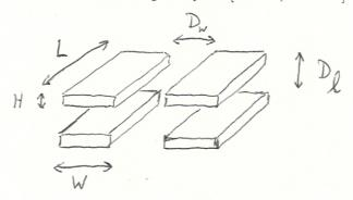
The time it takes a minimum transistor to drive a wire of length L, width W and thickness H can be estimated as follows. The wire is assumed to have distance  $D_l$  to neighbouring layers and  $D_w$  to other wires in the same layer. If  $W_0$  is the minimal width of a wire in the current technology, then the minimal transistor, consisting of a wire crossing, occupies area  $W_0^2$ . The total time T to drive a wire is approximated by:
