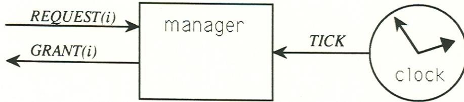
Figure 2: The architecture of the centralized control system.
