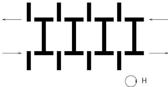
Figure 18: A double *TI*-bar track provides bidirectional propagation. Arrows show the directions in which bubbles propagate. The in-plane field *H* rotates counter-clockwise, as in Fig. 17
