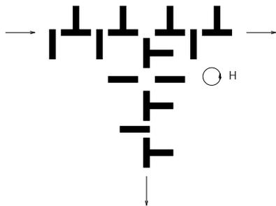
Figure 20: Bubble idler. The first bubble incident from the left is temporarily trapped in the circle of four permalloy conductors (*bottom center*). The second bubble incident from the left is prevented from making the right angle by its repulsive interaction with the trapped bubble. Simultaneously, the trapped bubble is freed, and along the downward track.
