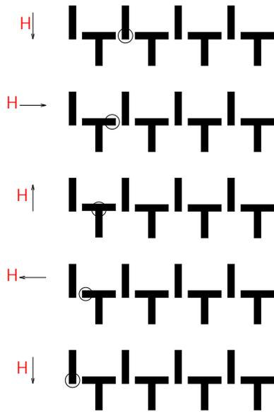
Figure 17: *TI*-bar track formed by permalloy conductors provides unidirectional propagation of the bubbles without changing their information-bearing state (i.e., their existence).
