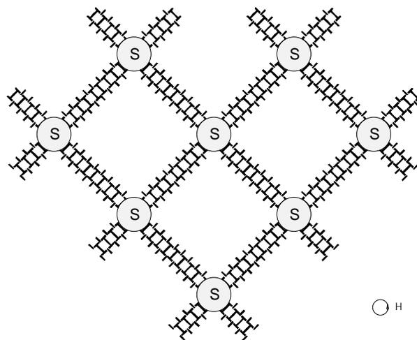
Figure 23: Permalloy circuit of a Few-Body cellular automaton that uses magnetic bubbles.
