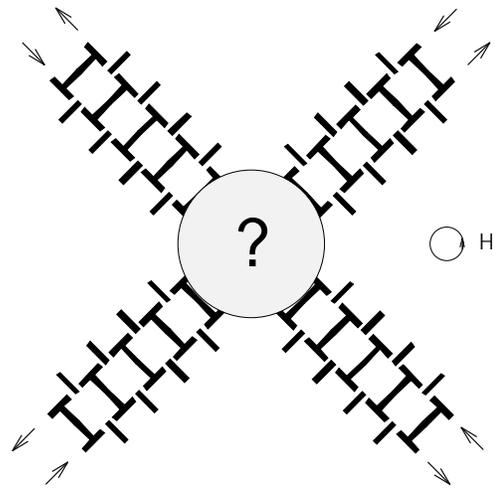
Figure 19: Can we replace the shaded “?” with some pattern of permalloy in such a way that it has the same 4-input/4-output logical function as the universal billiard ball rule of Fig. 11?
