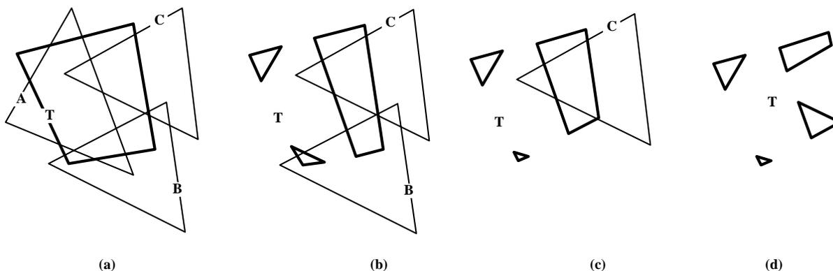
Figure 2: The figure shows a naive way of detecting occlusion. The polygons in Figure (a) are shown as they would appear in the image, *i.e.*, the reader is at the viewpoint. The occludee  $T$  is behind all the occluders  $A$ ,  $B$ , and  $C$ . Figures (b)–(d) show successive clipping of the occludee to each occluder to determine its visibility.
