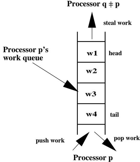
Figure 7: The per-processor load balancing work queue.
