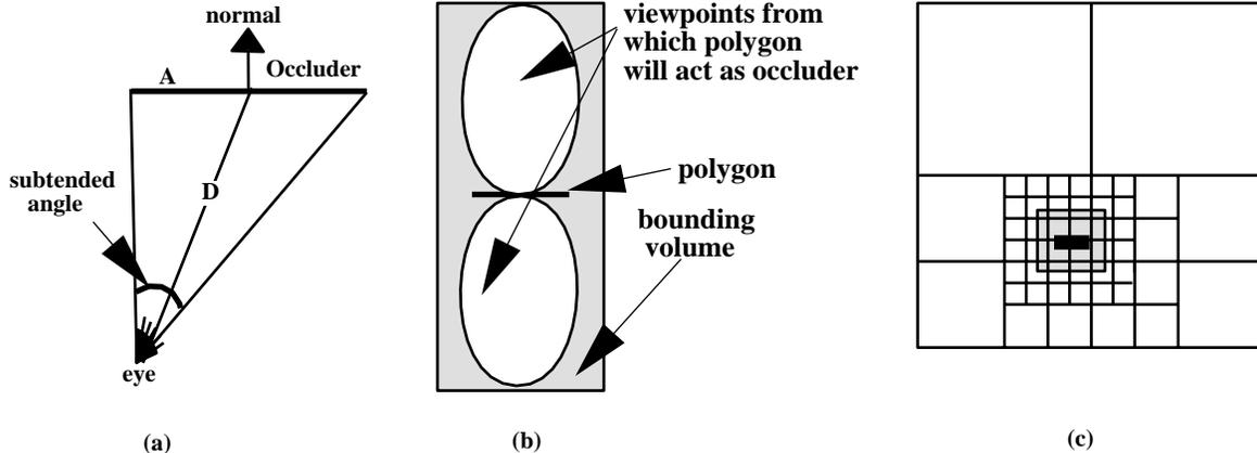
Figure 8: The subtended angle for a 2D occluder, and the components of the area-angle metric (a). The region of space in which the occluder is significant, i.e., where  $\text{area-angle} > \text{threshold}$  (b). Static insertion of an approximate occluder volume into the octree (c).
