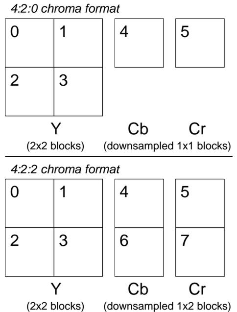
**Figure 7. Decoding stream to handle 4:2:0 and 4:2:2 chroma formats. Figures on right illustrate how macroblock orderings differ.**
