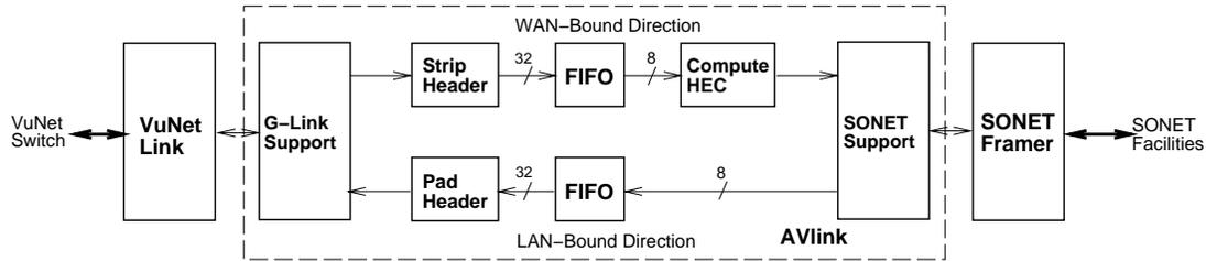
Figure 7: Block diagram of the AVlink
