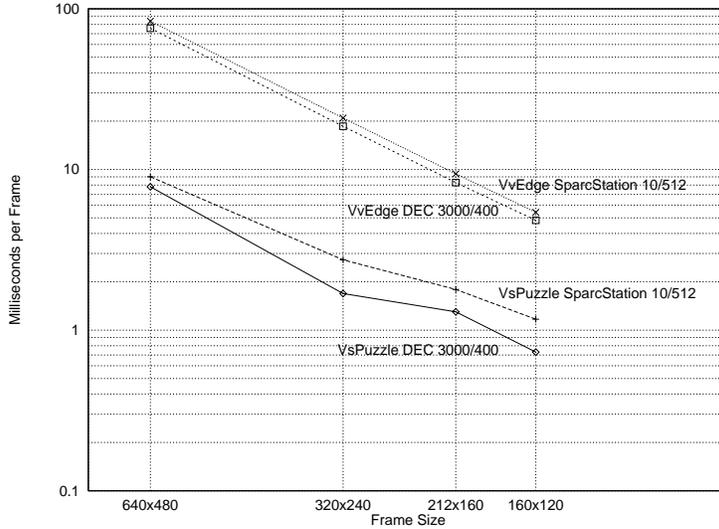
Figure 14: Processing Times of Representative Filter Modules.
