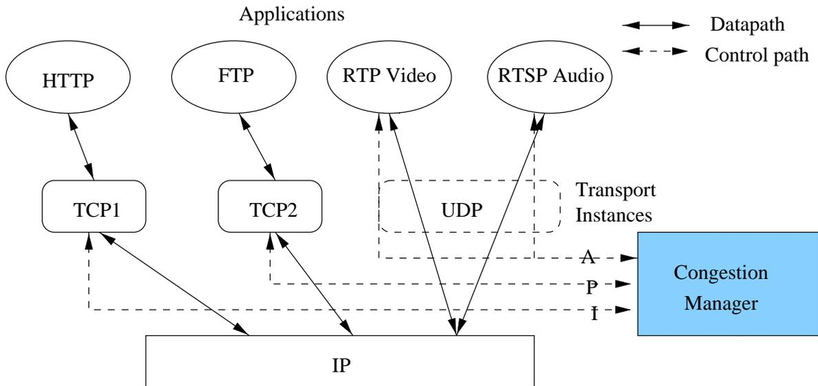
Figure 1: New sender architecture with centered around the Congestion Manager.
