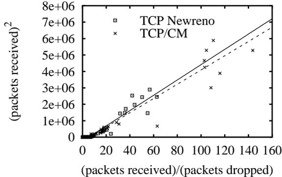
Figure 3: CM’s rate control is TCP-friendly.
