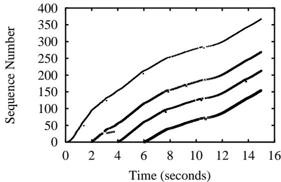
Figure 7: The CM scheduler apportions bandwidth well between simultaneous flows.
