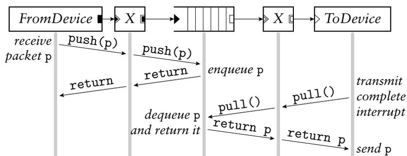
Figure 4: Functions called as a packet moves through a simple router. The central element is a *Queue*. During the push, control flow moves forward through the element graph starting at the receiving interface; during the pull, control flow moves *backward* through the graph, starting at the *transmitting* interface. The packet *p* always moves forward. The port colors indicate whether a connection is using push or pull processing: black means push and white means pull.
