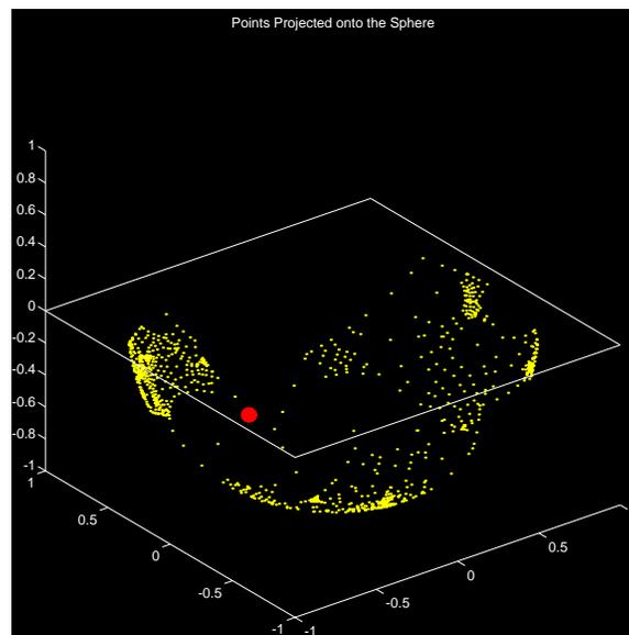
Figure 18.8: First we project the points stereographically from the plane onto a sphere (of one higher dimension than the mesh); Now we compute a "centerpoint" for the projected points in 3-space. Every plane through the centerpoint separates the input points into two roughly equal subsets. (Actually it's too expensive to compute a real centerpoint, so we use a fast, randomized heuristic to find a pretty good approximation.)
