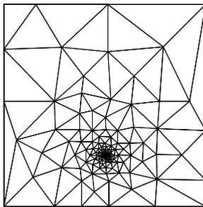
Figure 19.2: Triangulation of well-spaced point set around a singularity
