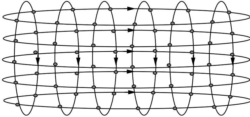
Figure 23.2: Embedding a Two-dimensional Grid in a Hypercube by bit-field partitioning.
