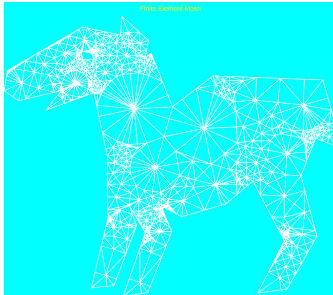
Figure 18.6: The input is a mesh with specified coordinates. Every triangle must be "well-shaped", which means that no angle can be too small. **Remarks:** The mesh is a subgraph of the intersection graph of a set of disks, one centered at each mesh point. Because the triangles are well-shaped, only a bounded number of disks can overlap any point, and the mesh is an "alpha-overlap graph". This implies that it has a good separator, which we proceed to find.
