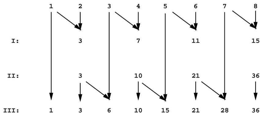
Figure 11.1: Action of the Parallel Prefix algorithm. The array in II comes from running `scan` recursively on the array in I.
