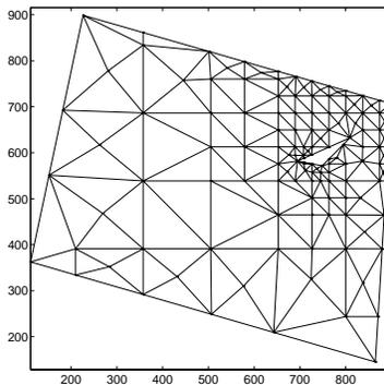
Figure 19.4: A well-shaped mesh generated by quad-tree refinement
