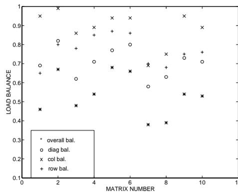
Figure 15.5: Efficiency bounds for 2-D cyclic mapping due to row, column and diagonal imbalances ( $P = 64$ ,  $B = 48$ ).
