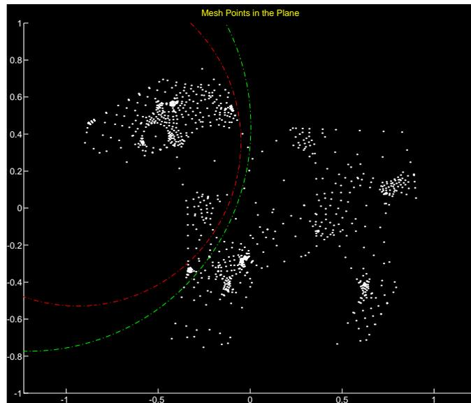
Figure 18.13: This partitions the mesh into two pieces with about  $n/2$  points each, connected by at most  $O(\sqrt{n})$  edges. These connecting edges are called an "edge separator".
