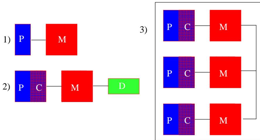
Figure 8.1: 1) A computer 2) A fancier computer 3) A multicomputer
