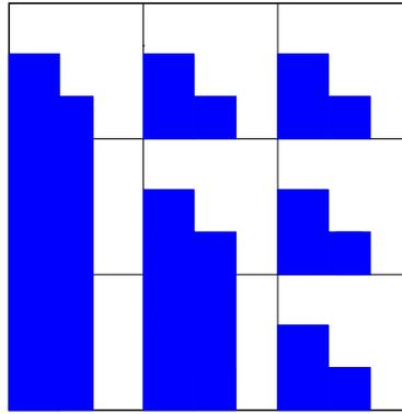
Figure 14.4: A stage in Gaussian elimination using cyclic order, where the shaded portion refers to the zeros and the unshaded refers to the non-zero elements
