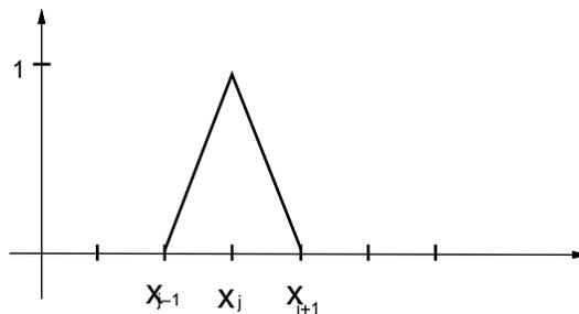
Figure 13.2: A basis function for 1D finite element
