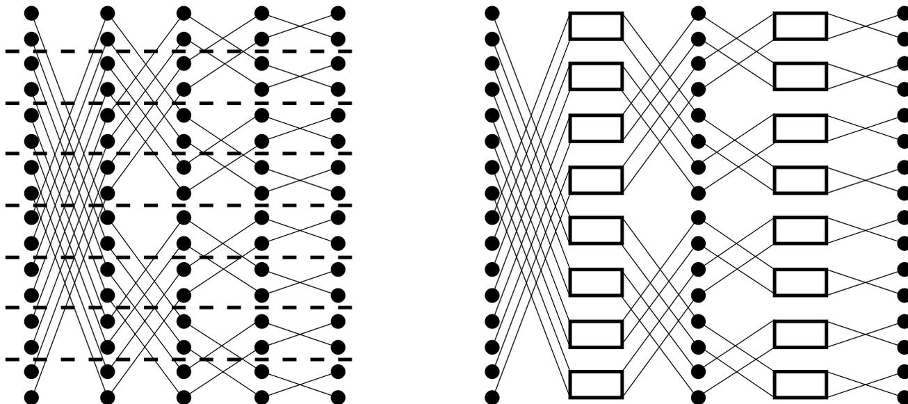
Figure 11.5: Left: more than one element per processor. Right: one box is a  $4 \times 4$  matrix multiply.
