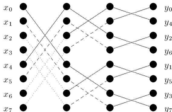
Figure 11.3: FFT network for 8 elements. (Such a network is not built in practice)
