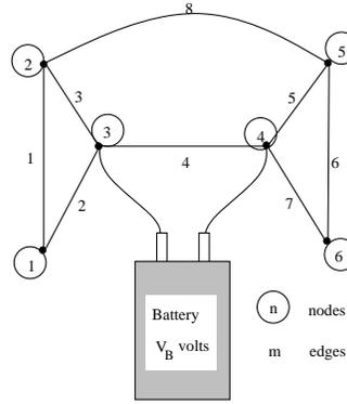
Figure 18.1: Resistor network with nodes and edges
