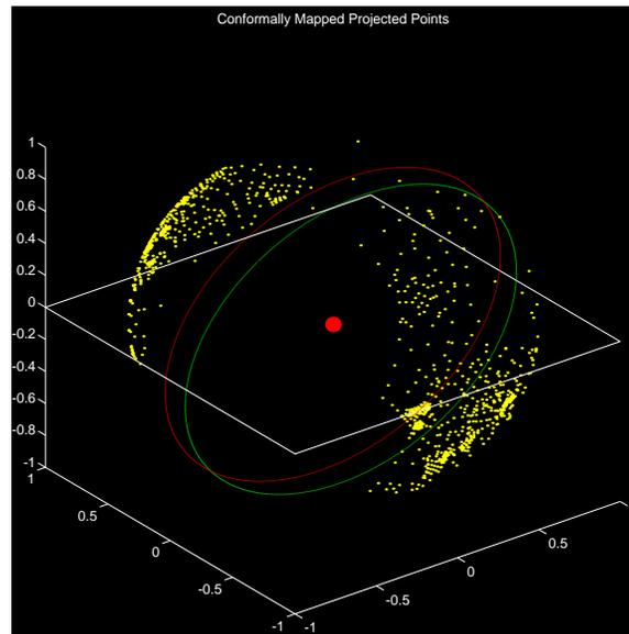
Figure 18.11: To translate this into a separator for the mesh, we first undo the conformal mapping, giving a (non-great) circle on the original sphere ...
