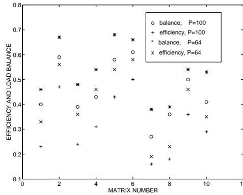
Figure 15.4: Efficiency and overall balance on the Paragon system ( $B = 48$ ).
