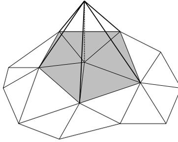
Figure 13.3: A basis function for 2D finite element
