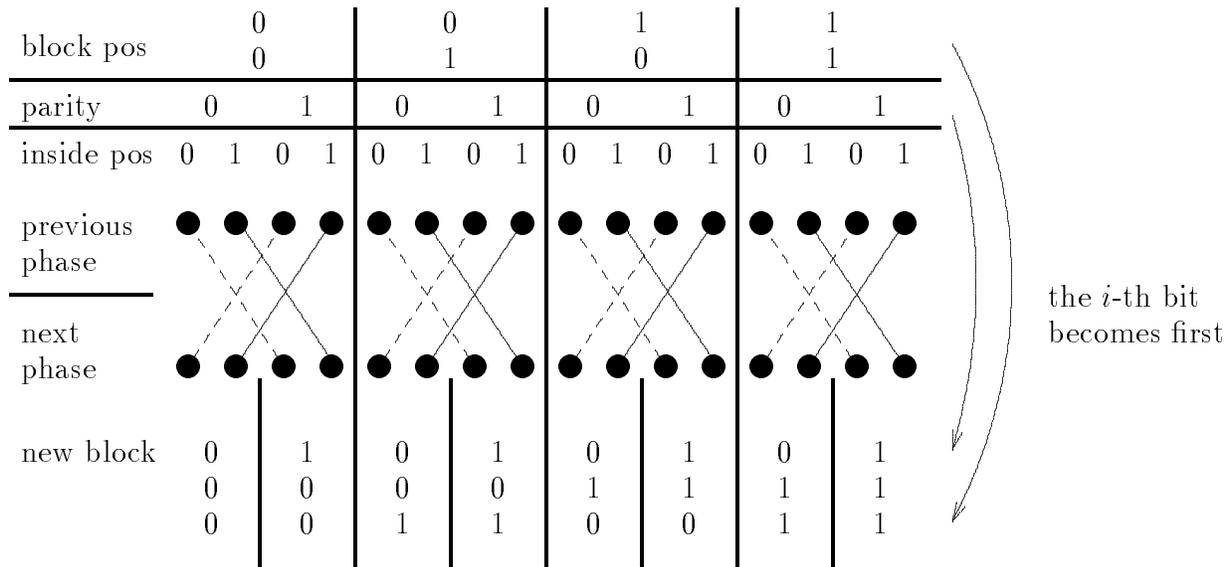
Figure 11.4: The output of FFT is in bit-reversed order.
