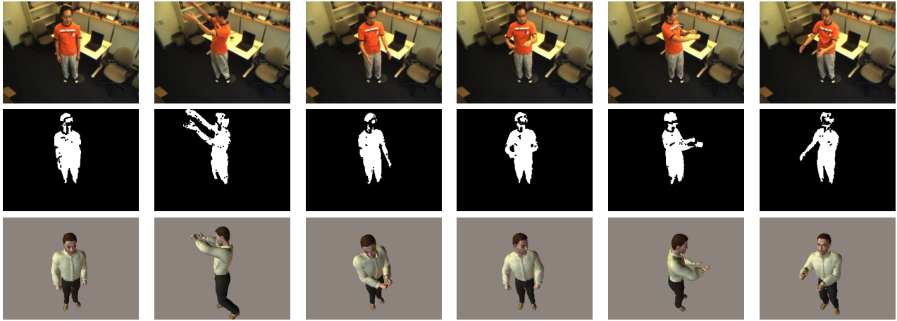
Figure 4: Sample frames from a gesture sequence (first row), segmentation masks (second row) and the corresponding frames from a most likely sequence computed by CRPV algorithm (third row). See supplementary material for the full video.
