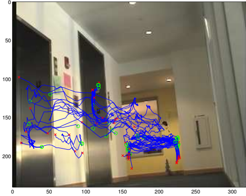
Figure 2: This figure shows con-trails for the tracking data of pedestrians in an elevator lobby. The tracks are blue and begin at locations with green circles and end at locations with red x's. There are three elevators in the left foreground. In the back, bottom of the image, one can see the hallway where many pedestrians pass from left to right or right to left. Though not visible in this camera view, there is a security door at the rightmost location where pedestrians exit.
